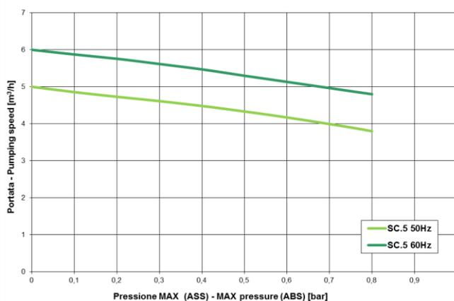
NOTE: Graph shows inlet pressure at a temperature of 20°C (tolerance ±10%)
